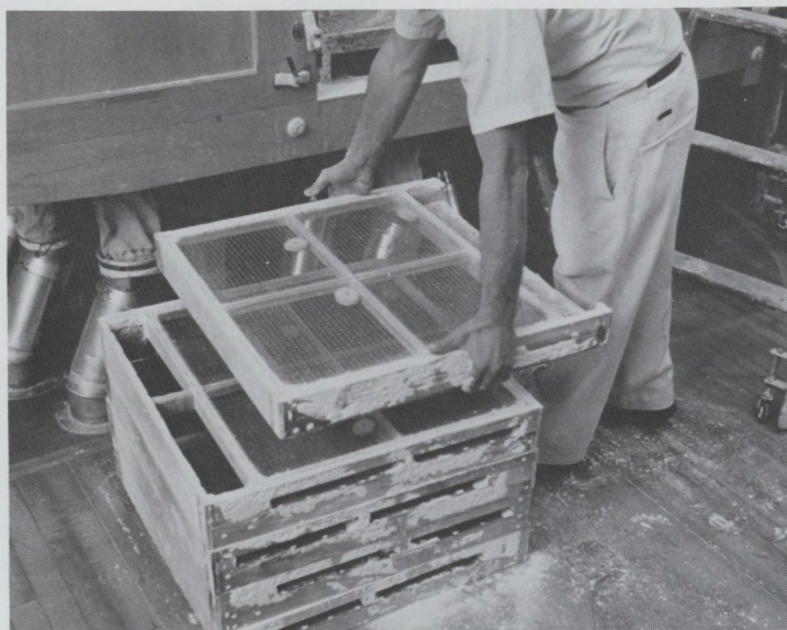
After wheat is broken into coarse particles at the roller stage, it is run through box-like sifters where it is shaken through a series of screens to separate the larger from the smaller particles. Photo Credit: Millers' National Federation
