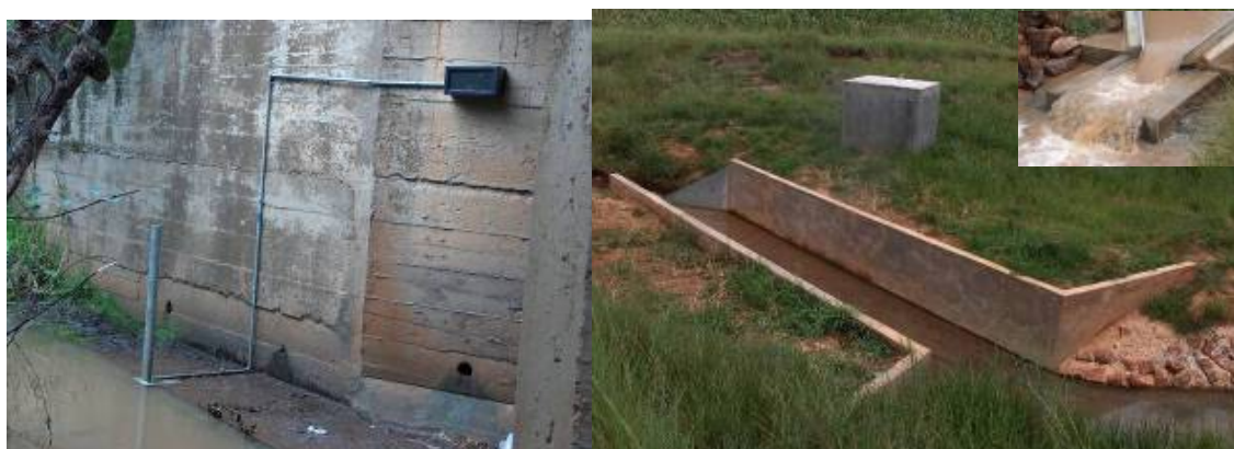
Figure 2.14: The Potshini H-Flume, and Pressure transducer at the outlet of the Potshini catchment.
