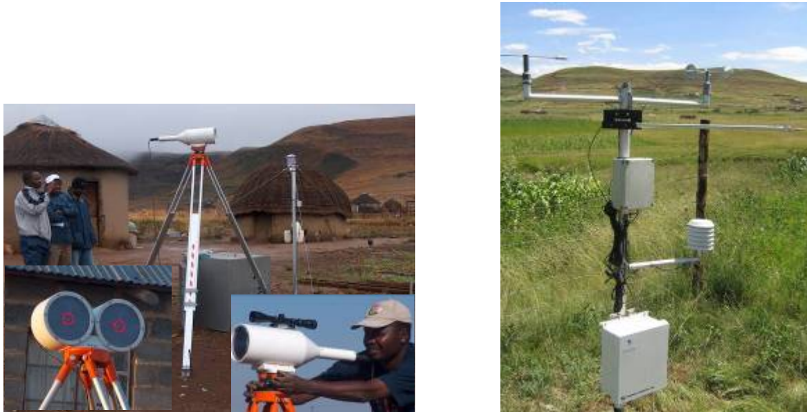
Figure 2.15: The Potshini Automatic Weather Station and Large Aperture Scintillometer.
