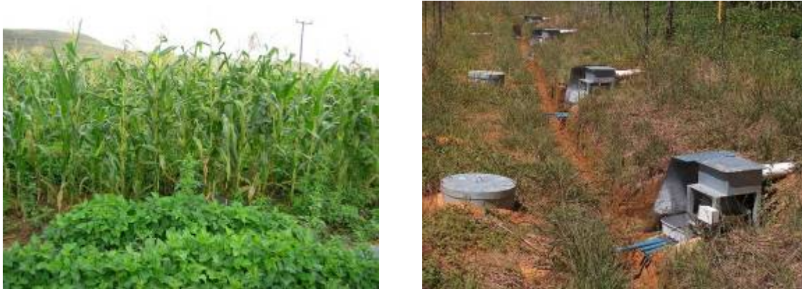
Figure 2.8: Communal trial site (researcher-managed) – runoff plots, tipping buckets, splitters and sediment load sampling tanks.
