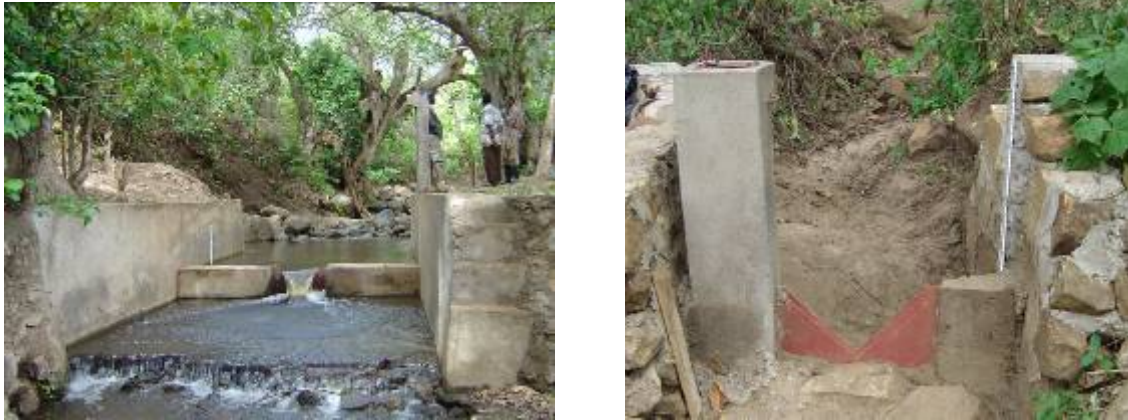
Figure 2.11: Runoff measurements in Makanya catchment.
