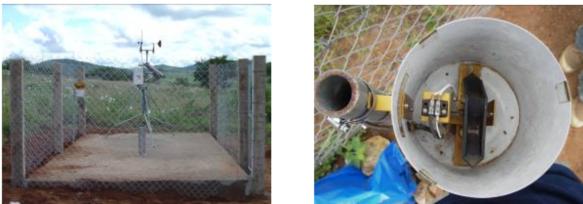
Figure 2.12: The meteorological station at Bangalala and an automatic rain gauge.
