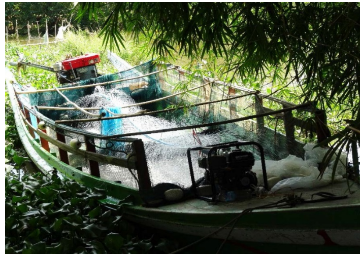
Specially modified fingerling transport boat with oxygenated 'live well'
