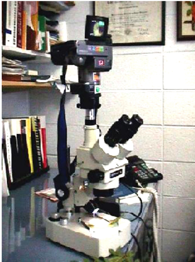
Figure 3. Compound Microscope Equipped with a Digital Camera for Use in Distance Digital Diagnosis.
