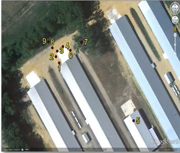
Figure 1. Soil Sampling Location at the New Poultry House (Site I): (1) 2 nd poultry house facing from back right side surface; (2) 2 nd poultry house side edge deep (10cm); (3) 2 nd poultry house front edge deep (10cm); (4) 2 nd poultry house front edge surface (5cm); (5) Manure storage pile located inside the storage shed; (6) 2 nd poultry house side edge surface (5cm); (7) Drainage swale between houses 3 and 5; (8) Before grass buffer strip; and (9) After grass buffer strip.
