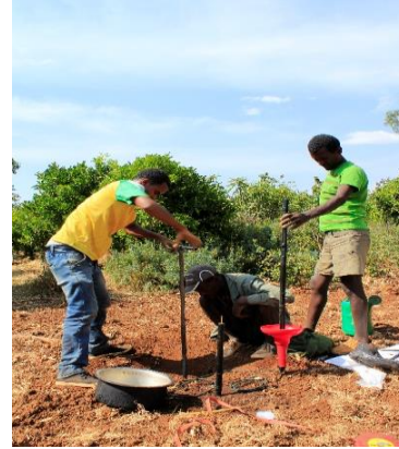
Figure 2 Installation of wetting front detector and access tube.
