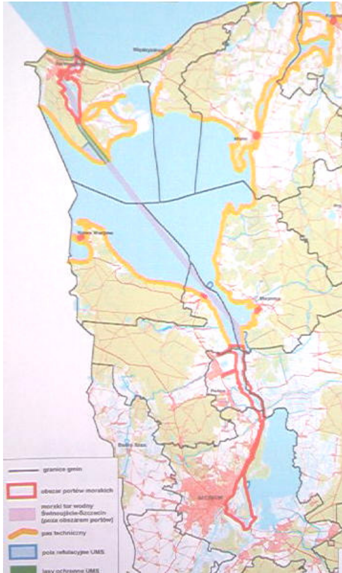
Figure 6 Map of fairway for shipping between Szczecin-Swinoujscie ports on Odra estuary (West pomerania) explanation for fig. 6, red outline – port area under Marine Office (UMS) management, light violet wide line - fairway
