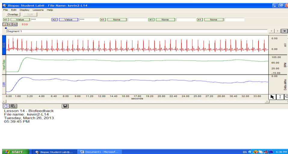
Figure 5. Example of a screen showing a measurement session. ECG is shown in the upper part of the screen, HR at the middle, and EDA at the bottom part of the screen
