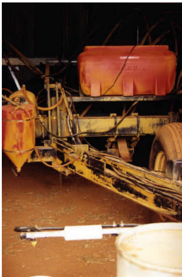
Figure 77 – Seeder with chemical application tanks fixed to frame. Orange indicates trifluralin use.
