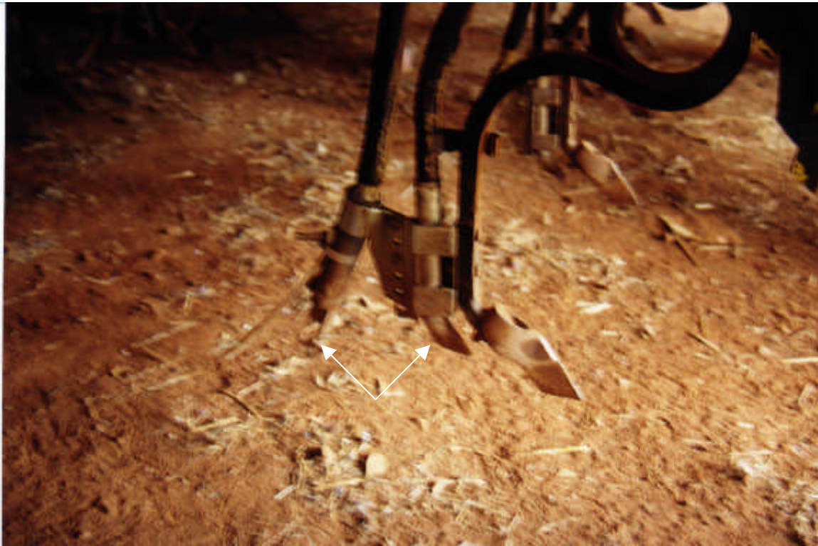
Figure 79 – Seeding equipment on present airseeder. Note seed tube and soil closer plate following deep knife point and fertiliser tube.
