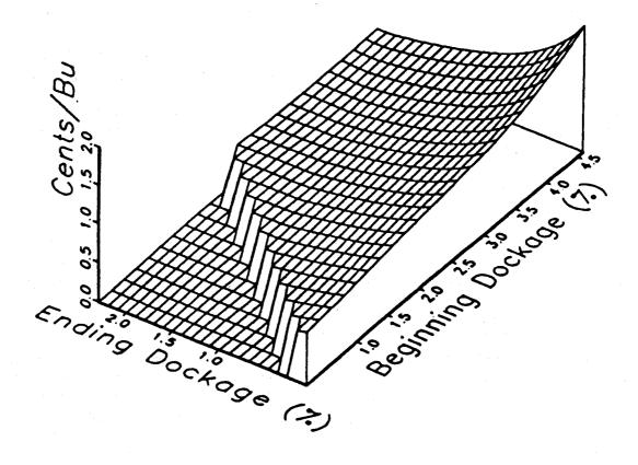
Figure 2: Disk-Cylinder Operating Costs Operating costs are estimated at \$5.05 per hour.<sup>9</sup> This includes costs of electricity, labor, and replacement parts for the disk-cylinder cleaner. It does not include depreciation or opportunity costs of capital. Extra handling costs (HC) are assumed to be zero.<sup>10</sup> Figure 2 displays operating costs on a per-bushel basis. Per-bushel costs depend on operating efficiency and, hence, on beginning and ending dockage levels.
