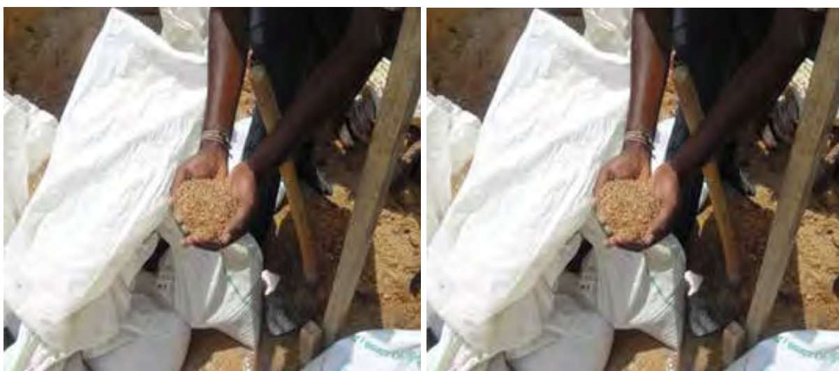
Figure 11.2.9. Gravel pack and installation.
