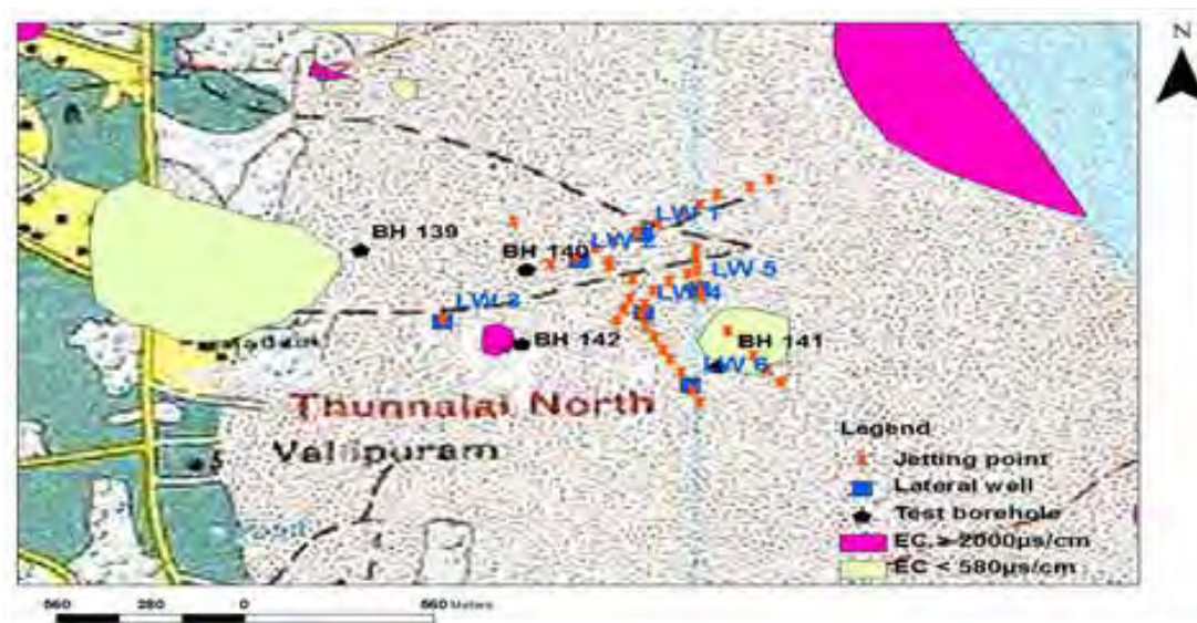
Figure 11.2.6. Proposed lateral wells with jetting points.
