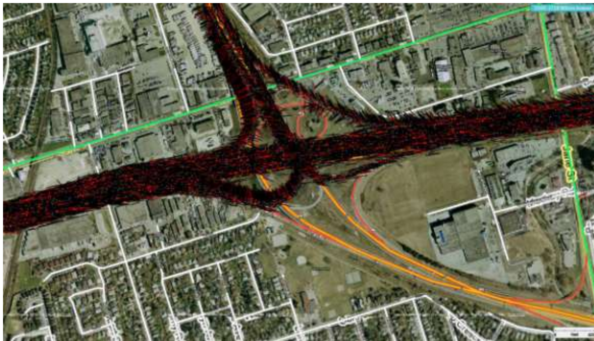
Figure 16, Geographic display of GPS data including a heading vector whose length is proportional to the speed assigned to the point. Data for Jan. 2008 at the intersection of the MacDonal-Cartier Freeway (ON 401) and ON 40.
