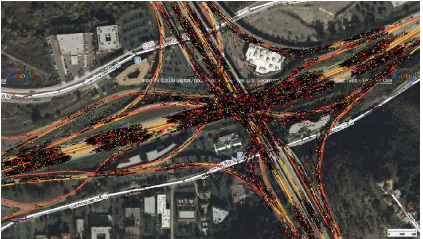
Figure 11, Display of only the most centered GPS point for each vehicle traversal of each arc of ALK's digital map database at the intersection of I8 and I 805 near San Diego, so-called "OneMon" data set.
