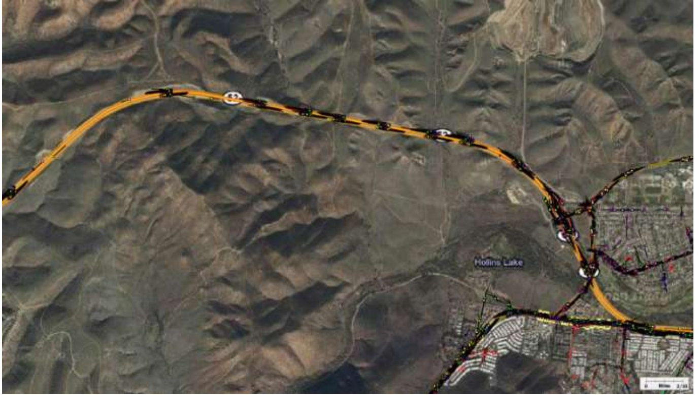
Figure 12, Display of only the most centered GPS point for each vehicle traversal of each arc of ALK's digital map database along CA 53 in Southeast California, so-called "OneMon" data set.
