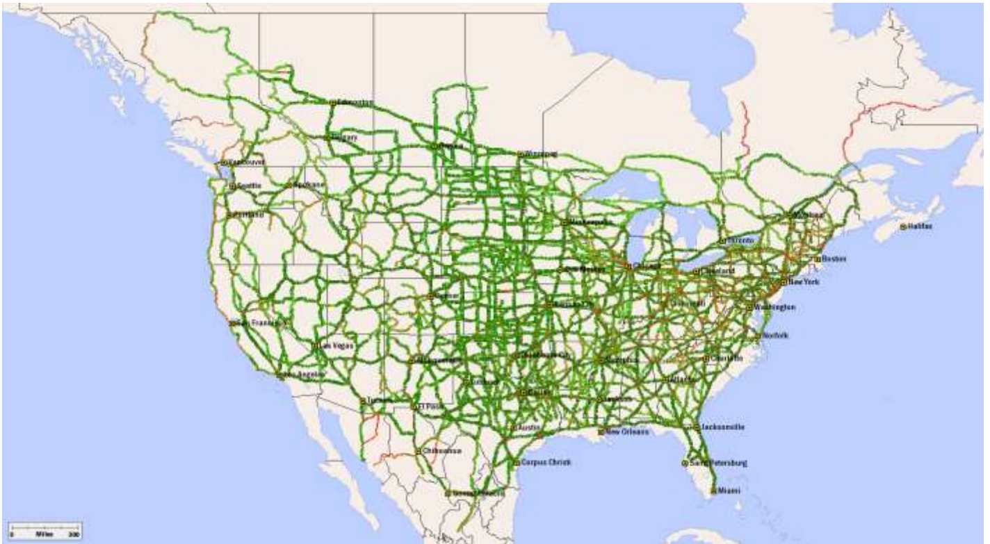
Figure 31, Display of Median Speed along the major highways in North America, as observed from ALK's GPS probe vehicle dataset.
