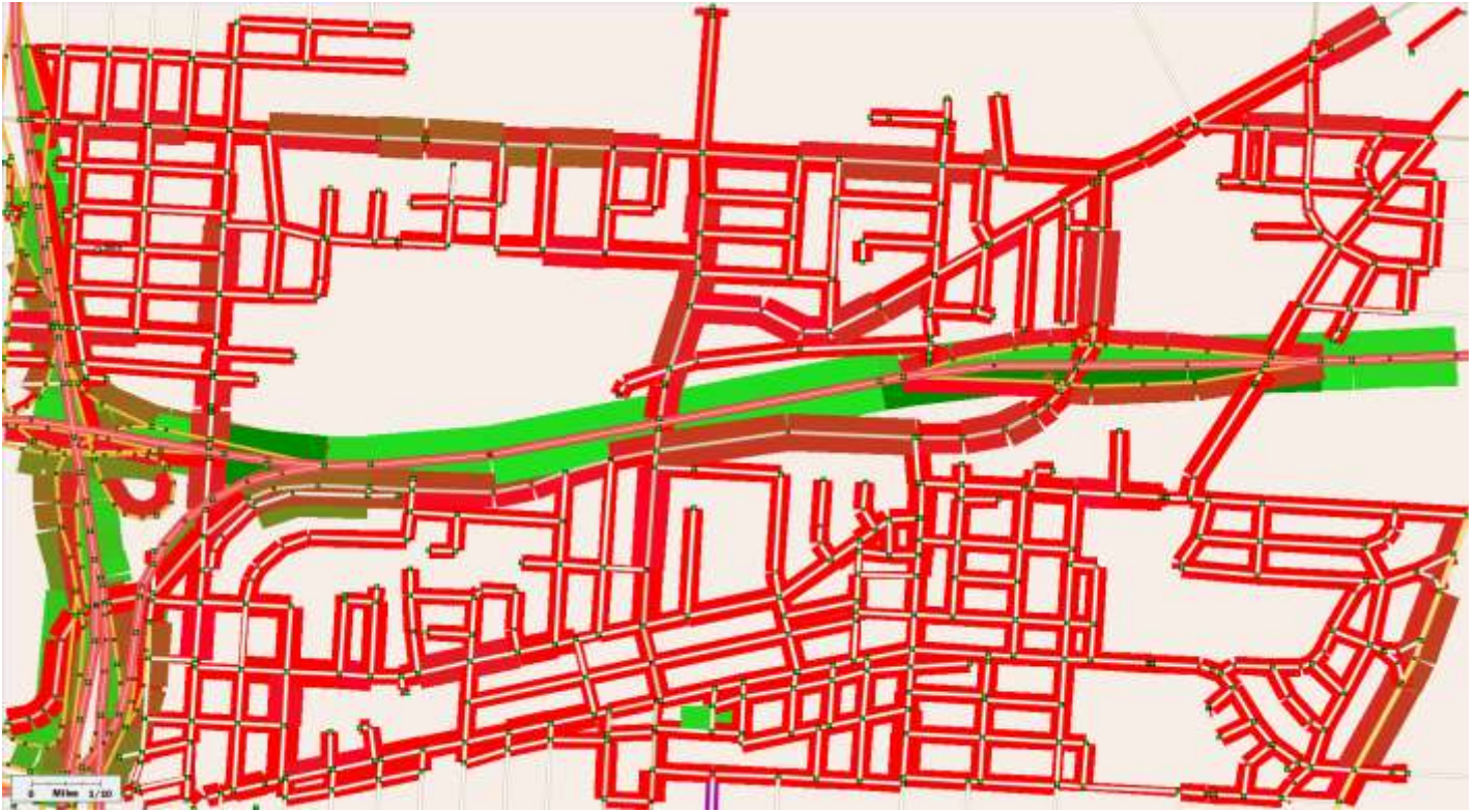
Figure 37, Display of Median Speed along all streets near the intersection of I-71 and I-670 Northeast of Columbus, OH as observed from ALK's GPS probe vehicle dataset
