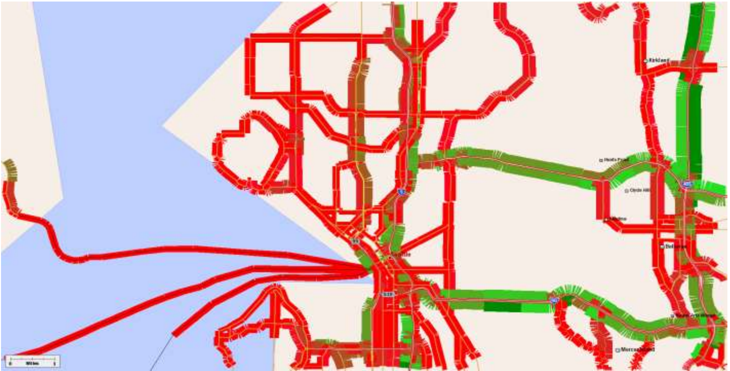
Figure 38, Display of Median Speed along all major and minor roadways near Seattle, WA as observed from ALK's GPS probe vehicle dataset
