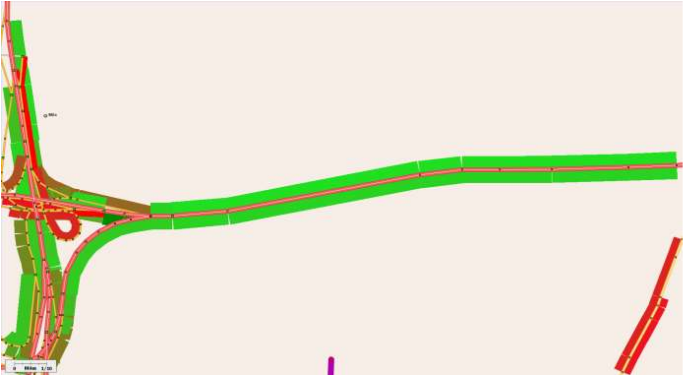
Figure 36, Display of Median Speed along the major highways near the intersection of I-71 and I-670 Northeast of Columbus, OH as observed from ALK's GPS probe vehicle dataset.
