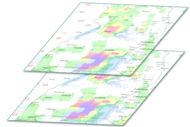
One day of gridded rainfall becomes a single gridded layer in the database.
