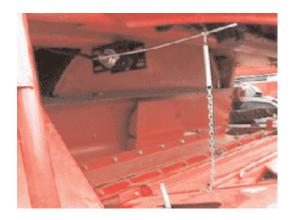
The rotor should be cleaned out from the front and sides by opening existing access covers
