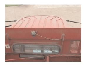
Combine sieves should be pulled to facilitate clean out and reentry of grain. One-way nuts and long bolts can be added to ease alignment and replacement.
