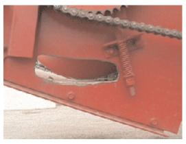
A hole is cut in one end of the header to blow grain out. Operators simply take an air hose, start in the far end and blow grain across the table and out the exit hole. It is difficult to blow the grain out of a header without the hole because wind in the corner catches kernels deflecting them back into the header. Vacuuming is difficult because it is difficult to reach completely around the auger.
