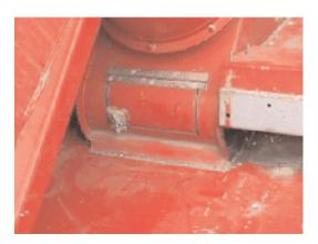
In addition, all exposed ends of sheet metal and corners should be caulked to prevent kernel lodging.
