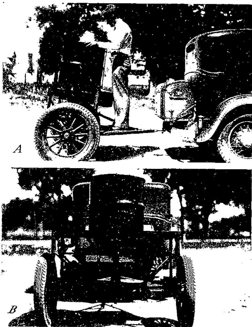
FIGURE 4.—Mechanical spreader for grasshopper bait, Colorado, 1936: A , Side view; B , rear view.
