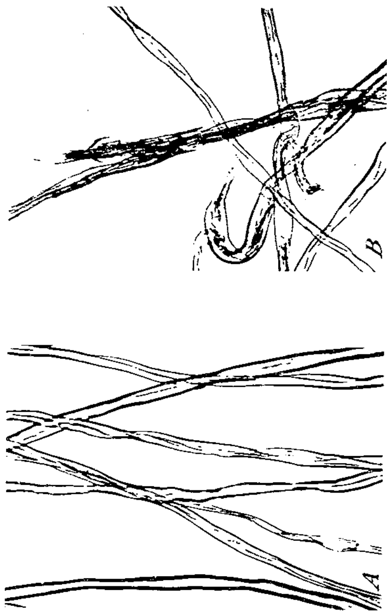
Fibers stained with basic fuchsin: A , Untreated fibers; B , fibers removed from the fabric incubated for 15 days with Charcotomium glabosum . \times 250 .
