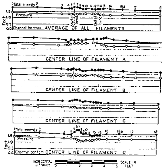
FIGURE 41.—Pressure and total energy gradients for four equal filaments of flow in a 180° bend with a 5-inch inner radius. Channel 5 inches wide by 10 inches deep. Discharge 1.88 cubic feet per second.
