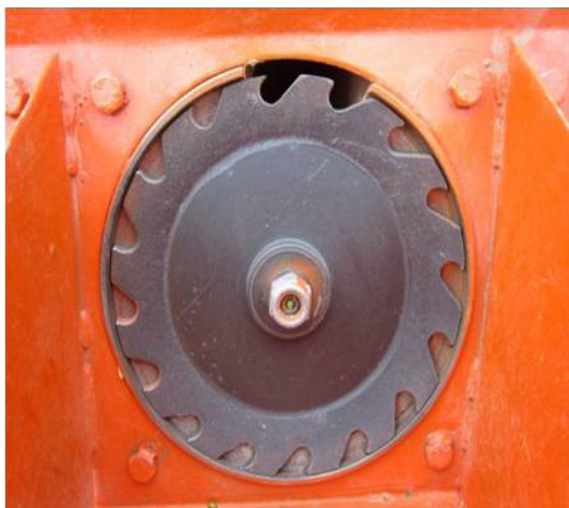
Plate 7. Seed-metering systems used for dry seeding of rice.
