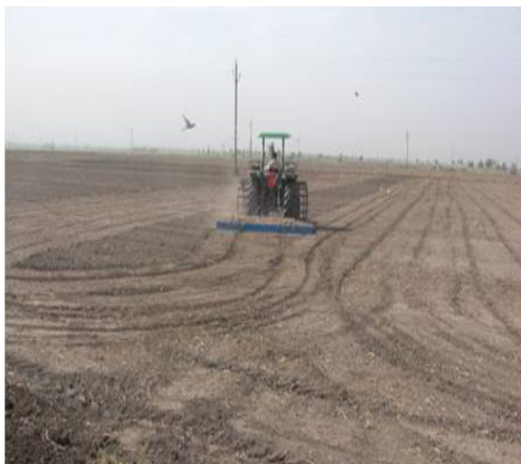
Plate 5. Land leveling using metal board and laser land leveling.
