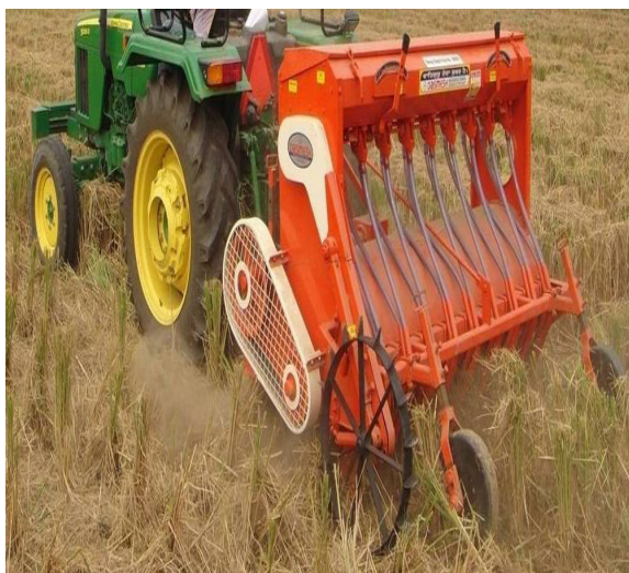
Plate 10. Seed drills capable of seeding in high residue amounts.
