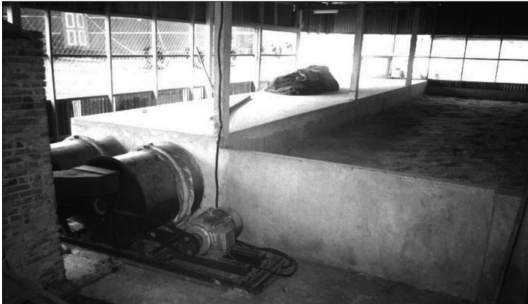
Fig. 4. Rice husk furnace with vortex and central-pipe ash-precipitation chamber.
