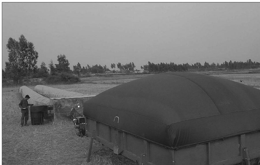
Fig. 9. The SDG-4 dryer using solar heat; a top cover is used for downward airflow.
