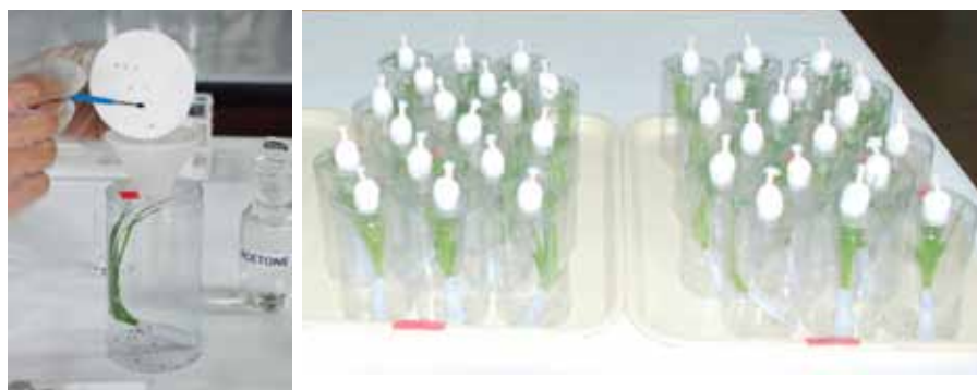
Fig. 5.6. Treated planthoppers are transferred into clear tumbler cages through a funnel.
