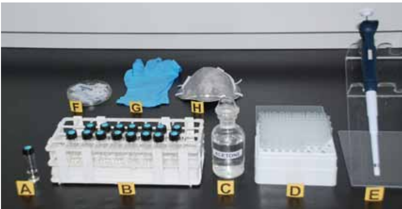
Fig. 5.2. Materials for preparation of serial dilutions: (A) stock solution, (B) 6-mL screw cap vials with label, (C) technical-grade acetone, (D) pipettor tips, (E) pipettor, (F) parafilm strips, (G) disposable nitrile gloves, (H) disposable mask.
