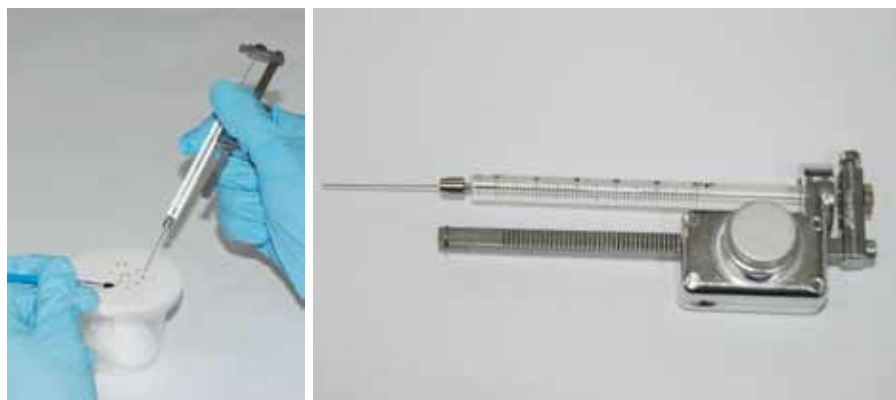
Fig. 5.5. Topical application: (A) anaesthetized planthoppers on watchglass wrapped with gauze; (B) Hamilton Repeating Dispenser and microsyringe.
