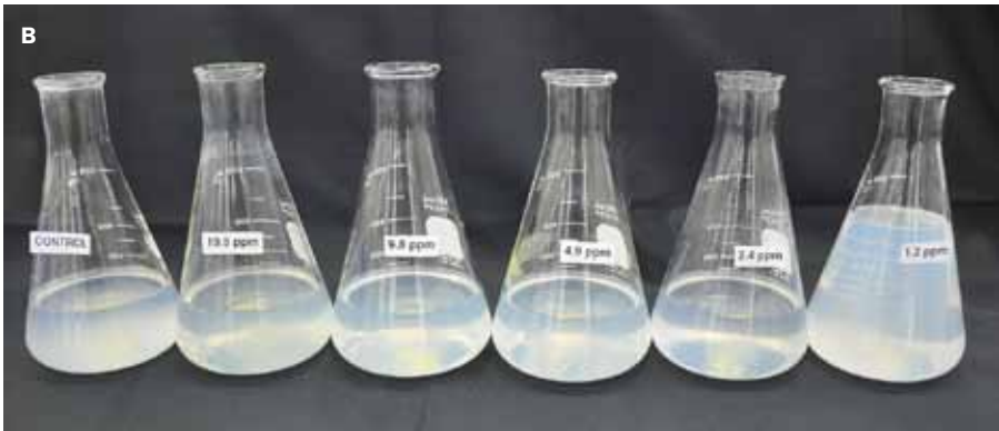
Fig. 9.1. Preparation of stock solution: (A) technical grade insecticide dissolved inside a standard volumetric flask; (B) Erlenmeyer flasks with insecticide dilutions.
