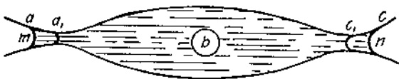
FIGURE 11.—A capillary tube of nonuniform bore, with a bubble of entrapped gas: a , One aperture; a_1 , position of minimum radius of aperture a ; b , a bubble of entrapped air or other gas; c , the other aperture; c_1 , position of minimum radius of aperture c ; m , meniscus at aperture a ; n , meniscus at aperture c .
