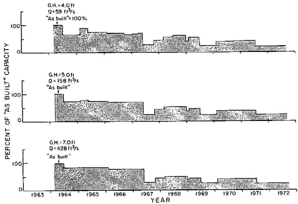
FIGURE 3.12.—Discharge rates as a percentage of as-built capacity for selected stages, watershed W-A2 (1964-72).
