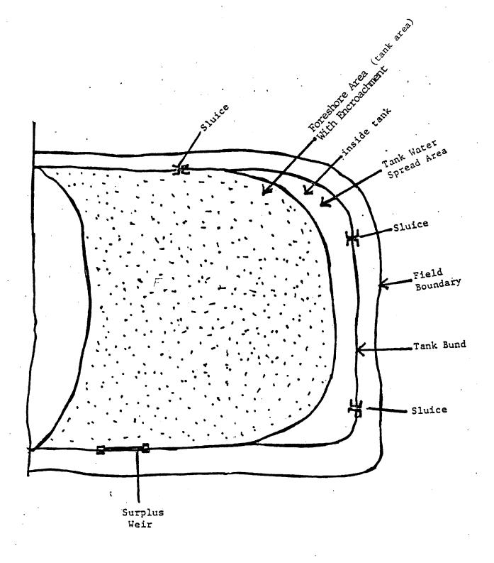
FIGURE 1. Tank with Severe Encroachment and Sedimentation.
