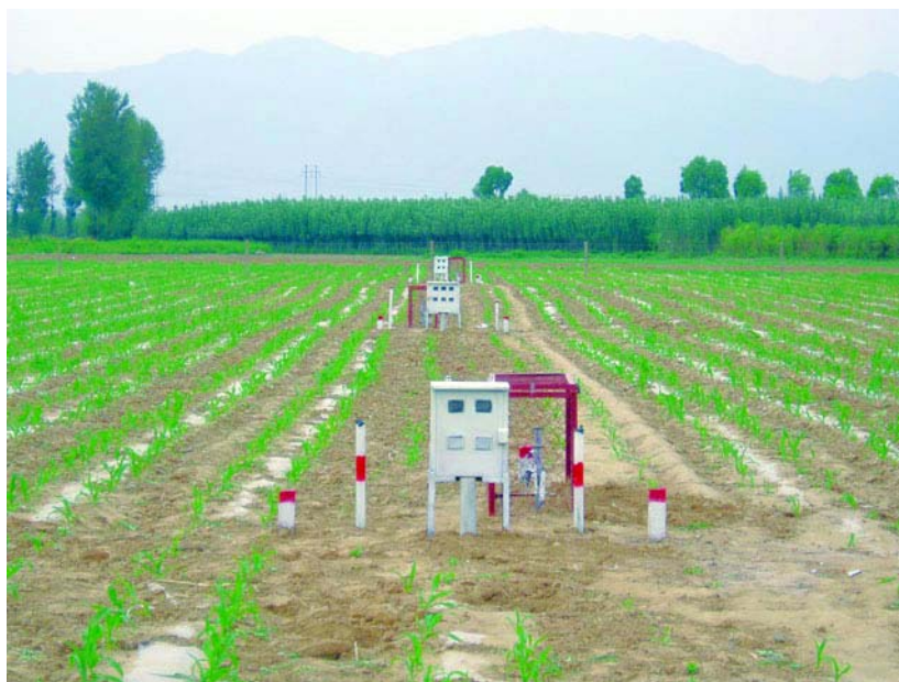
Figure 6. FILTER trial site in Da Tong, Shanxi Province showing terminating boxes, cages over tensiometers and soil suction samplers in the plot in the foreground. The three terminating boxes can be seen on the three plots. The cabling between these terminating boxes and through to the data logger is buried.
