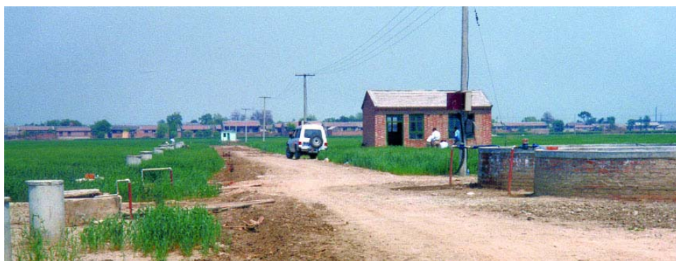
Figure 5. FILTER trial site in Wuqing, China. The subsurface drainage from the FILTER plots located on both sides of the centre road collects in the drainage sumps (located in a row adjacent to the road) and is then pumped to the drainage storage tank (right foreground)
