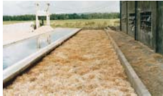
Figure 3. Soaking of wood-wool to remove water soluble extractives
