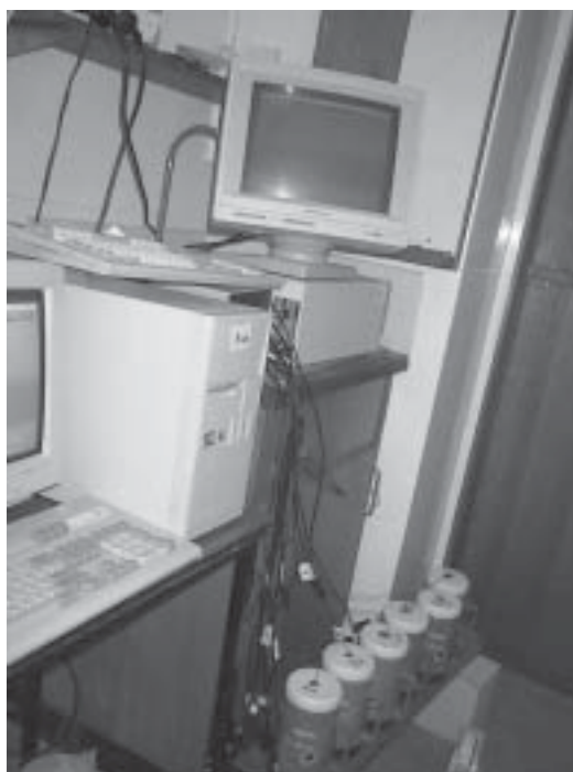
Plate 3. Hydration temperature-logging apparatus in controlled climate room
