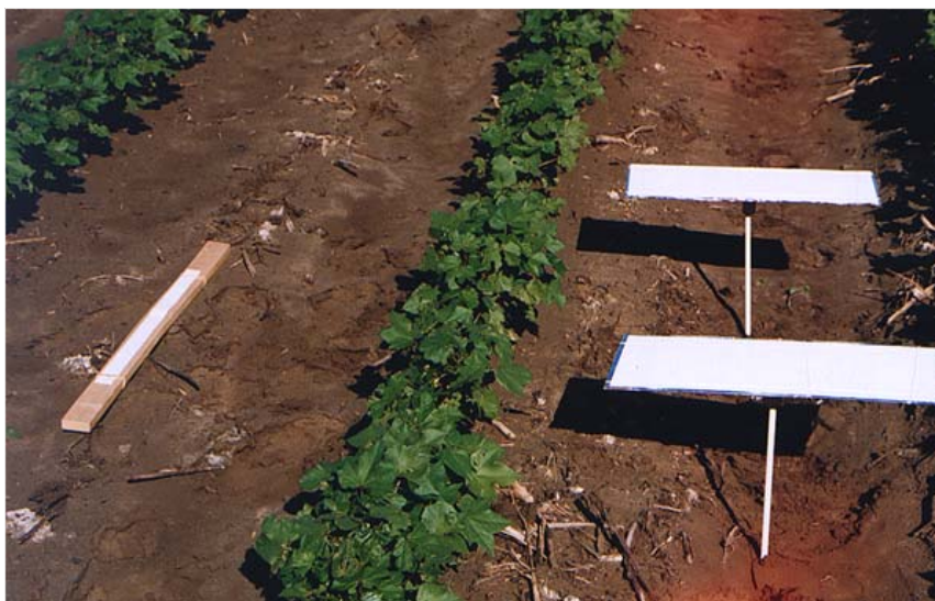
Figure 3. Plates and slats used to verify chemical application and deposition rates on cotton fields. Filter papers were extracted with acetone, and endosulfan estimated by GLC and ELISA analyses.
