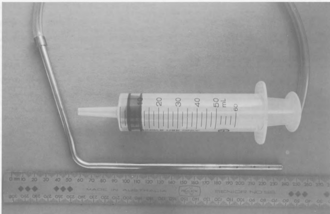
Figure 3. Apparatus used to collect parotid saliva from sheep.
