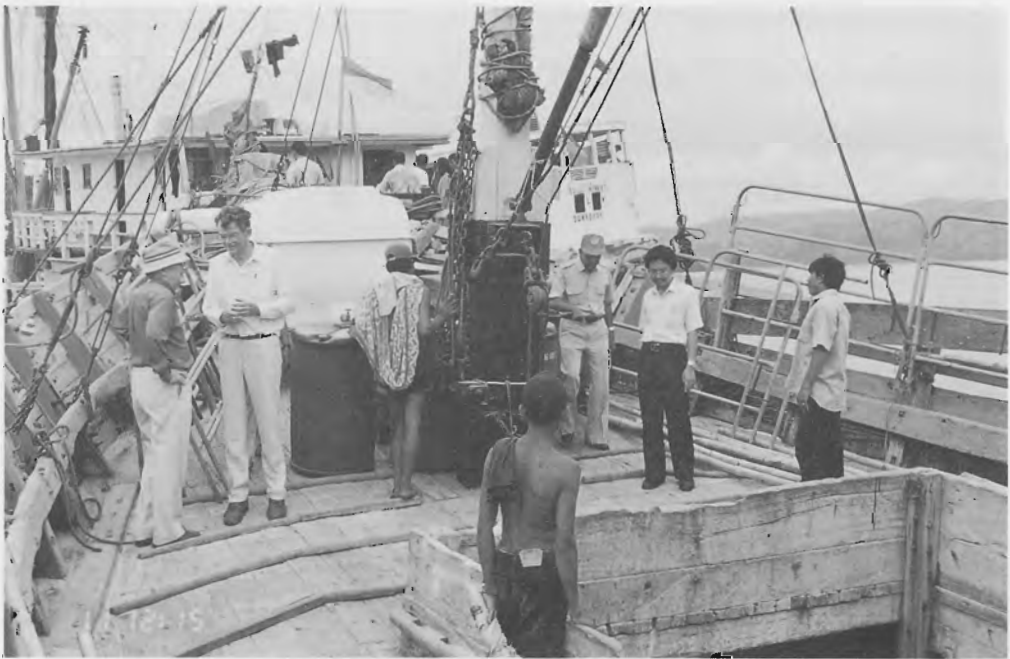
Figure 3. A modified Indonesian motorised sailing vessel before being set up for the receipt of cattle. A large water tank is evident in the forward part of the vessel with some portable panels along the sides.
