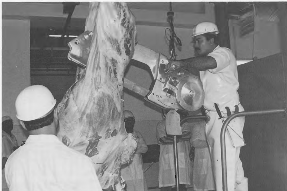
Figure 11. Use of the carcase splitting saw at the Senawang abattoir in Malaysia.
