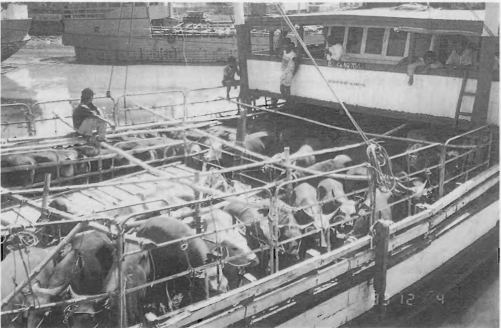
Figure 2. A modified Indonesian motorised sailing vessel on arrival at Surabaya with a load of cattle. The portable panels are used but have been supplemented by some bamboo rails. It is not possible to see the feeding troughs or the water supply.
