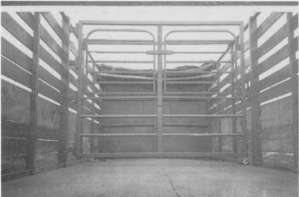
Figure 7. The modified livestock crate with the second deck removed for the transport of cattle in Indonesia.
