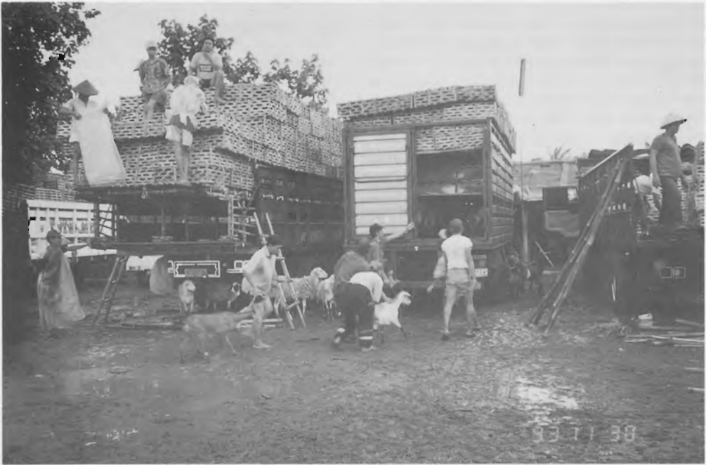
Figure 6. Goats being loaded on to the lower deck of the multipurpose livestock crate with chickens in bamboo crates on the upper deck. A traditional Indonesian truck was being loaded alongside the modified truck.
