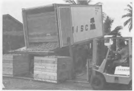
Fig. 4. Simple hopper for unloading bulk oranges.
