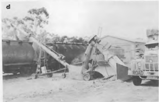
Fig. 8. Various views and uses of the grain auger (screw conveyor): (a) rear view of extractor auger; (b) extractor auger used to outload grain from silo and elevating auger to load it into rail wagons; (c) extractor auger as used for outloading grain from a shed; (d) extractor and elevating augers filling rail wagon from temporary (portable) road dump pit; (e) extractor auger used for feeding grain to belt slinger for pad storage filling.
