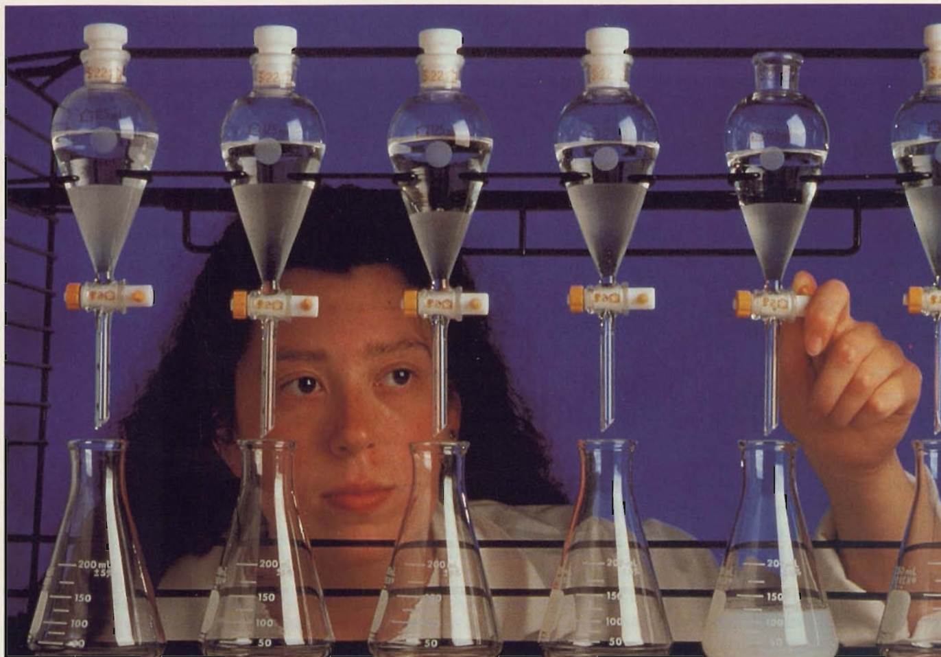
Biological laboratory technician Elizabeth Denvir extracts samples for total lipid and fatty acid composition.
