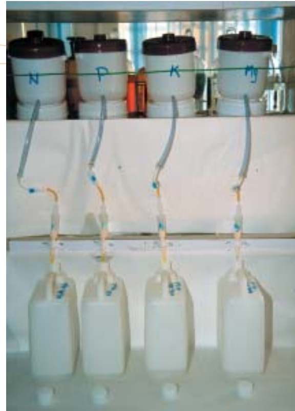
Figure A3.1 Purification of macronutrient salts for omission trials at the National Institute of Soils and Fertilisers, Hanoi, Vietnam. Note use of blood transfusion drippers to regulate the flow of solution from the reservoirs to the resin columns.
