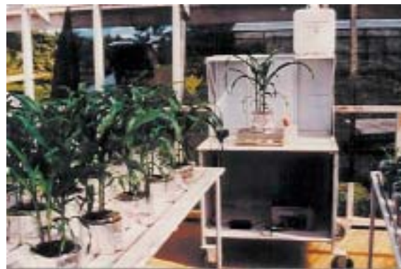
Figure 2.3 View of a portable weighing table showing deionised water bottle (top right), digital balance and pot (centre), and 240 V AC power inverter connected to a 12 V car battery (bottom).
