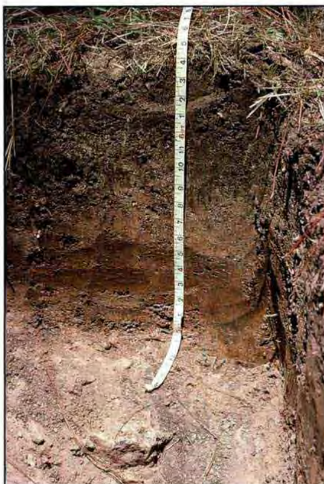
Shallow prairie soil; uniform nigrescent clay with prismatic structured melanised horizon, developed on basalt in a seasonal rainfall environment, restricted drainage when wet, droughty when dry (Mollisol). Reaction acidic tending alkaline with depth. Plantation of Pinus caribaea , Koro, Fiji. Photo: D.I. Bevege, ACIAR
