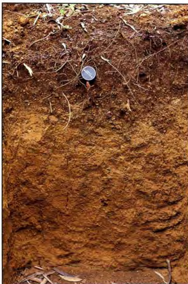
Well-drained lateritic Red Earth, gradational acidic profile with increasing clay and lateritic gravel with depth, some organic accumulation in A1 horizon and bleached A2, massively structured (Ultisol). Developed on sediments. Eucalyptus exserta plantation. Dongmen, Guang Xi, China. Photo: D.I. Bevege, ACIAR
