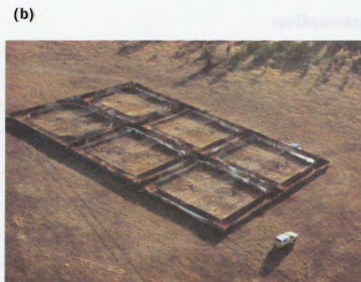
Figure 4. Outdoor enclosures used for manipulative experiments examining the effectiveness of fertility control to reduce mouse population abundance and rate of increase. Each enclosure is 15 m \times 15 m in area and is protected from predators by wire mesh fencing. Mice are prevented from burrowing into or out of the enclosures by metal fences that are buried to a depth of 800 mm. Food and water are provided ad libitum. (a) Ground-level view; (b) Aerial view.
