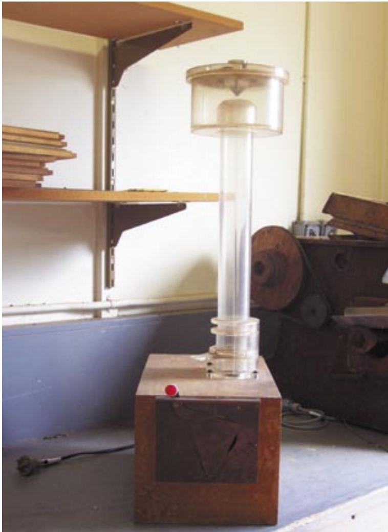
An aspirator used for cleaning seeds. Air is gently blown from a small fan in the base housing through the column, where dehusked seeds are collected in a sieve, while dust and husks accumulate in the top container.
