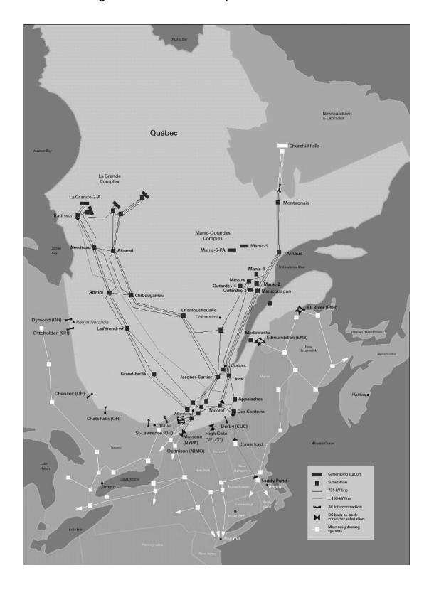
Figure 3. A simplified version of Québec's electric power network
