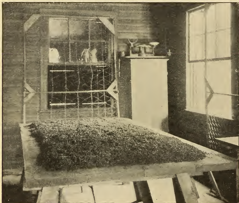
FIG. 6.—Method of oxidizing the rolled leaf. The wire screens when put into position hold up the damp cloths.
