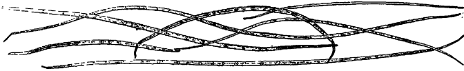
FIG. 17.—Rice-straw fibers. Though comparatively short, these are strong and felt well. (Enlarged 71 times.)
