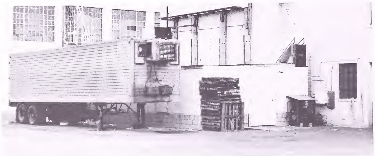
FIGURE 7.—Secondhand cooler and refrigerated trailer provide needed cold storage space with no protection from inclement weather.
