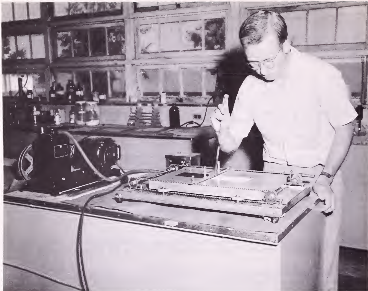
Figure 1. --Application of acetone solutions of experimental chemicals to kraft paper with an automatic blade applicator.
