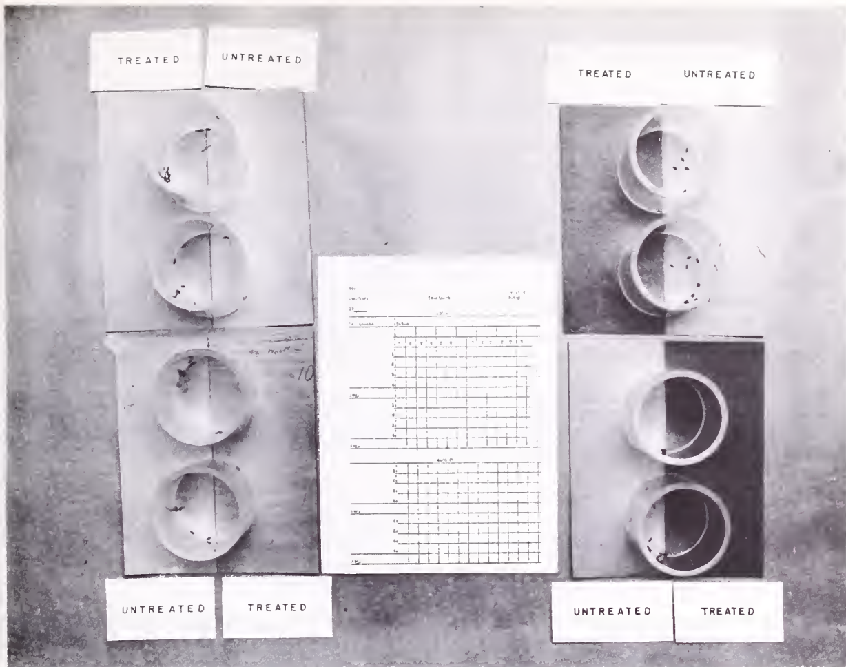
Figure 2.--Laboratory technique for determining the repellency to flour beetle adults of chemicals applied to kraft paper. Note test arenas composed half of treated paper and half of untreated paper.
