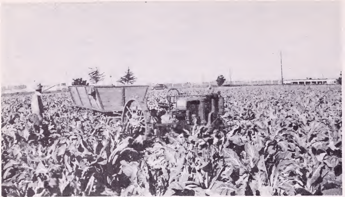
Figure 1.--Collecting cauliflower in the field. Operator sets tractor in slow motion and tosses heads into bin mounted on sled.
