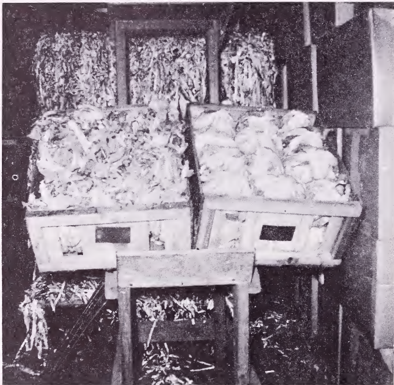
Figure 8.--A pony crate and a broccoli crate after examination. Note the disarrangement of the standard crate on the left compared with the orderly condition of the double-layer pack.
