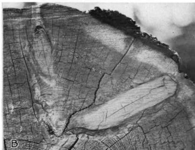
A, Cross section through a swollen knot. This is a detailed view of the swollen knot shown in Plate 4, A; B, cross section through sound knots. This is a detailed view of the sound knots shown in Plate 4, B. (Photographs by the writer and R. E. McArdle)
