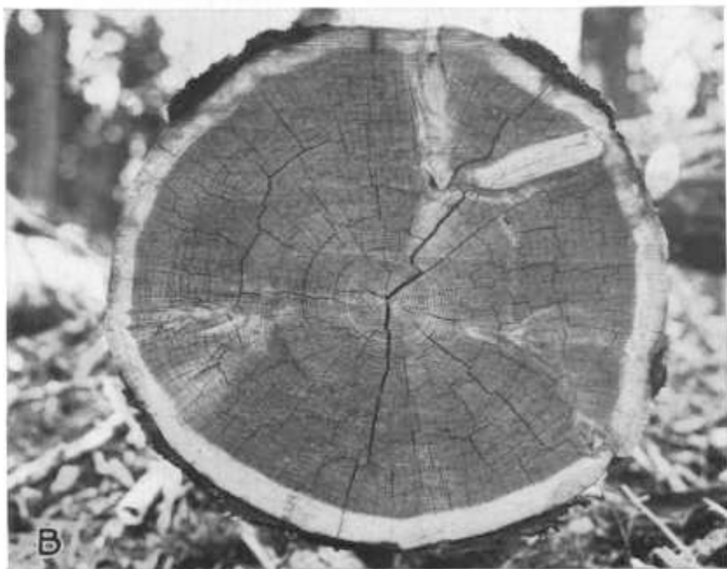
A, Cross section through a Douglas fir log with red ring rot caused by the ring-scale fungus, Trametes pini , showing a swollen knot; B, cross section through a sound Douglas fir log showing normal knots. (Photographs by the writer and R. E. McArdle)
