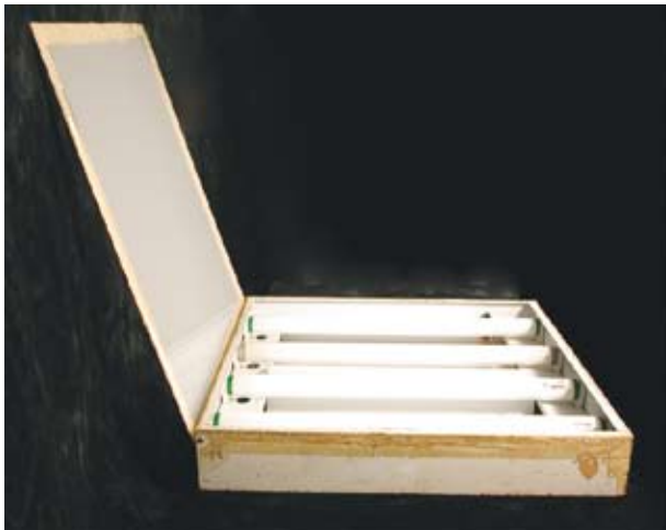
Figure 11. Side view of a type (b) light table with the top open.
