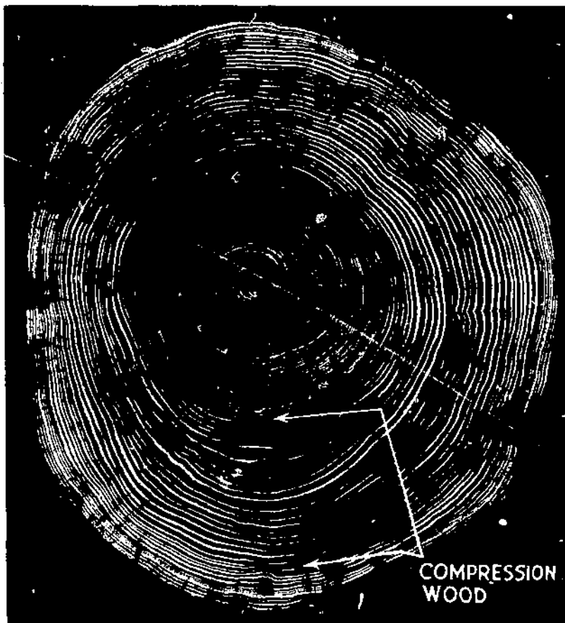
Cross section of a loblolly pine showing accelerated diameter growth and coincidental occurrence of pronounced compression wood following release by logging operation.
