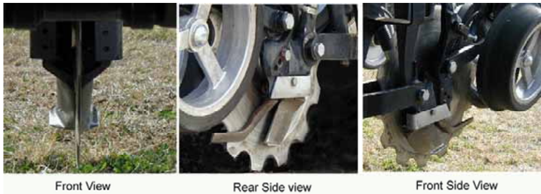
Figure 97: Front, rear and side views of the bioblade type furrow opener
