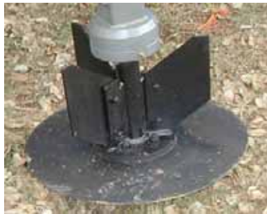
Figure 45: An example of a horizontal disc type row preparation device
