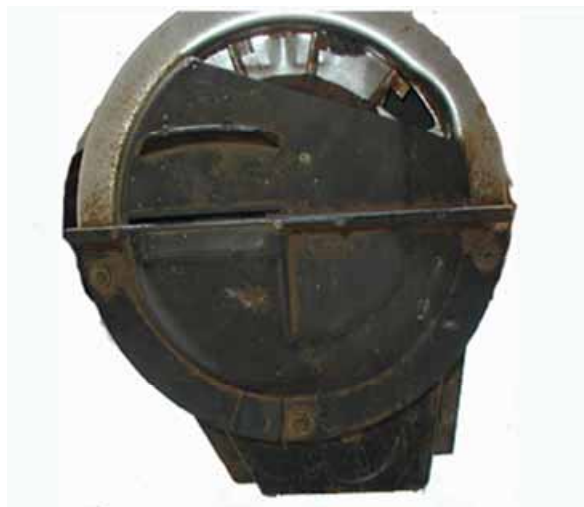
Figure 199: An example of a finger pick-up type precision seed meter
