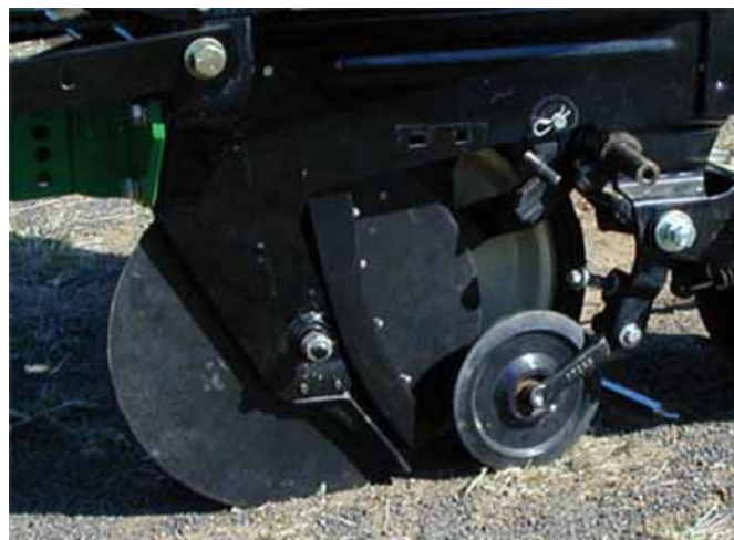
Figure 69: A typical seed placement device for use with single disc coulters type openers
