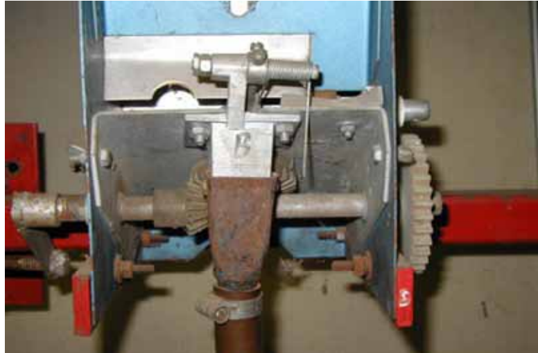
Figure 180: the rear view of an inclined plate type seed meter
