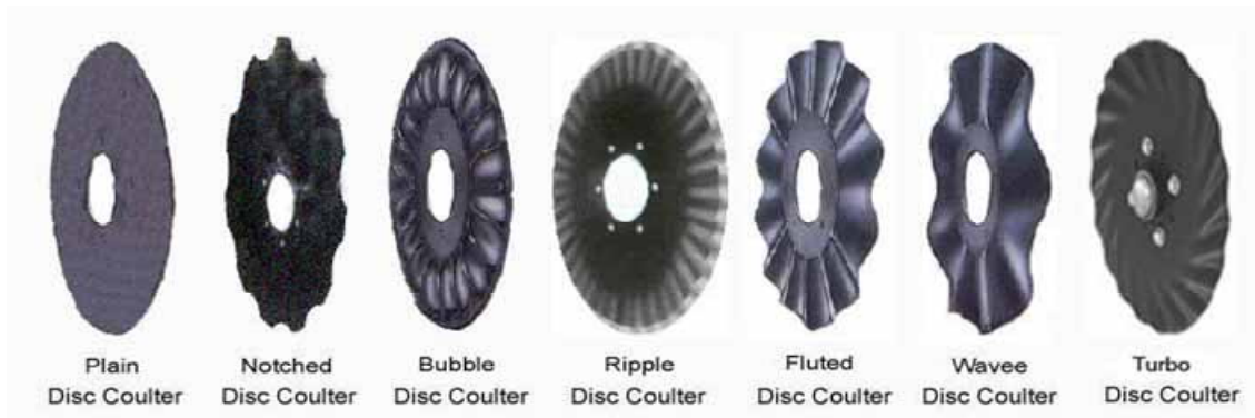
Figure 16: Types of disc coulters soil and residue cutting devices
