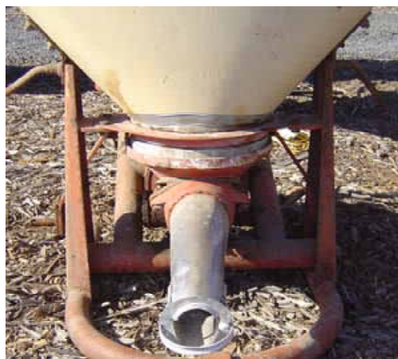
Figure 205: Oscillating spout type of mechanically assisted delivery system
