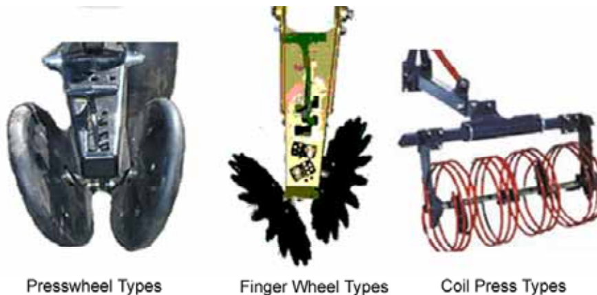
Figure 123: Types of seedbed firming devices
