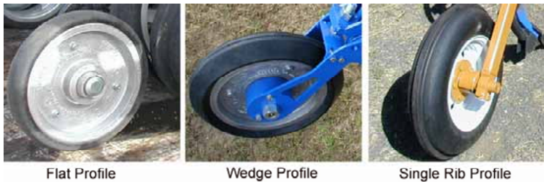
Figure 126: Some types of over-centre press wheel profiles
