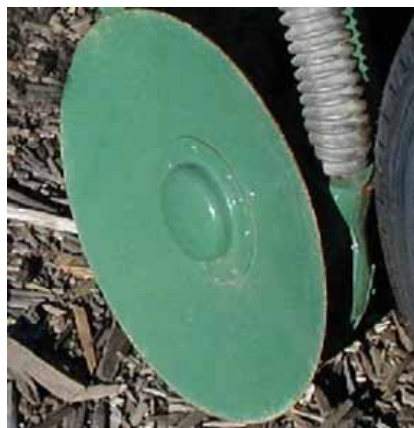
Figure 55: A single concave disc type furrow opener (rear side view)
