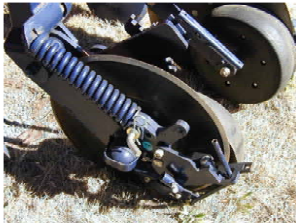
Figure 161: A dedicated gauge wheel type of the trailing arm system of depth control
