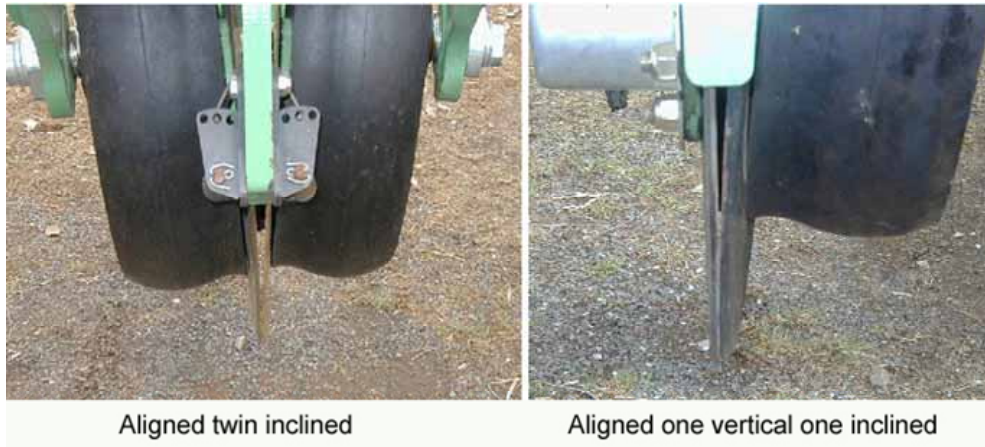
Figure 74: Aligned 'twin inclined' and 'one vertical-one inclined' types of double disc opener
