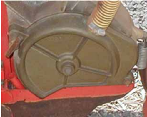
Figure 200: Seed delivery by gravity drop through the rear, split cavity of a runner opener
