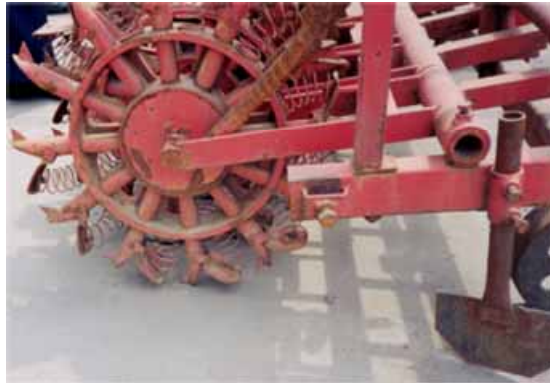
Figure 101: A punch type opener for planting through plastic mulch
