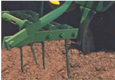
Figure 39: An example of a harrow type row preparation device
