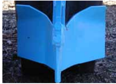
Figure 27: Example of a blade type row preparation device
