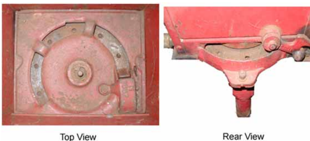
Figure 177: The top and rear views of a horizontal plate seed meter
