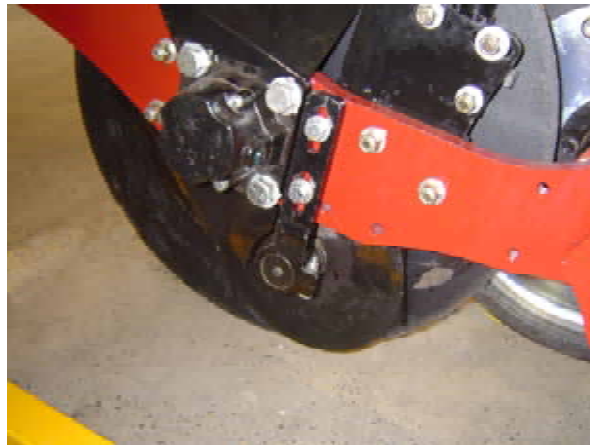
Figure 70: A rotary disc type seed placement device on a single-angle disc coultter opener
