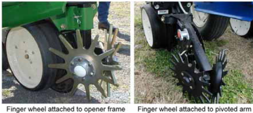
Figure 32: Spring steel finger wheel row preparation device
