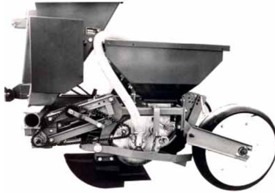
Figure 154: A unit planter utilising a 'rear gauge wheel' type of the parallelogram system
