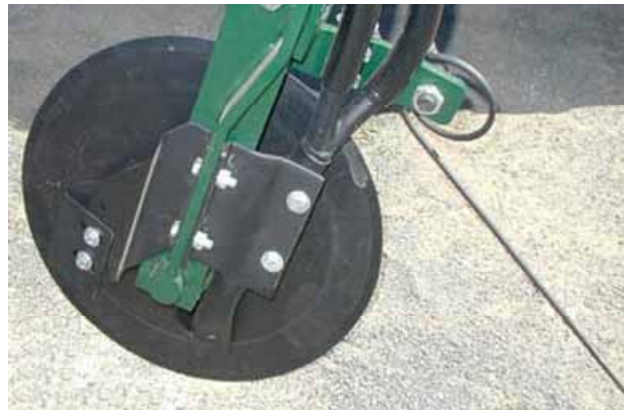
Figure 120: A single finger type covering device
