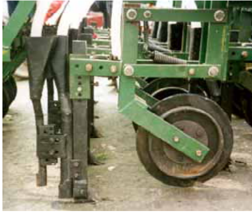
Figure 156: A furrow opener utilising a 'front gauge wheel' type of the parallelogram system
