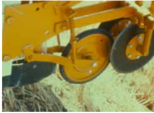
Figure 111: Double disc coulters type covering devices following a seed-firming wheel
