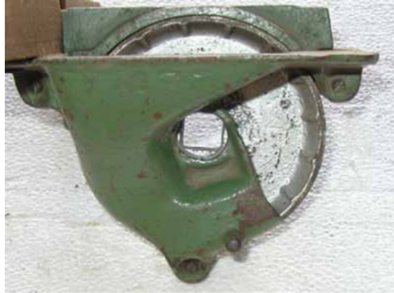
Figure 172: The side view of a typical internal force feed type seed meter
