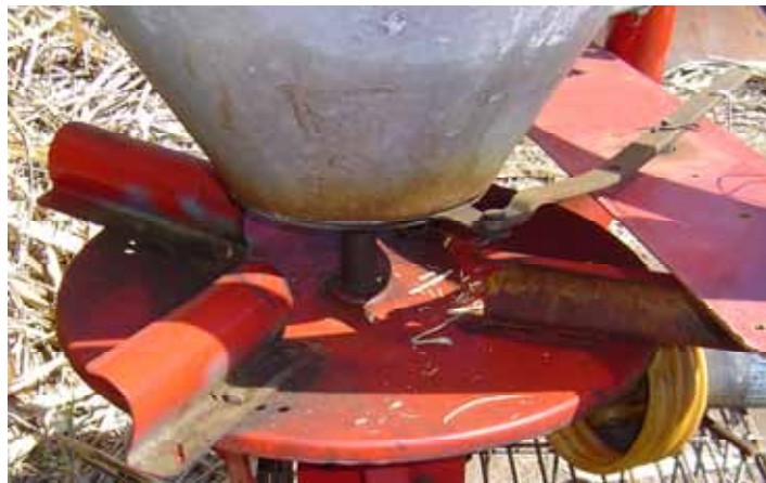
Figure 204: Spinning disc type mechanically assisted seed delivery system
