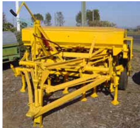
Figure 11: A 14-row, trailed, tractor-powered drill planter
