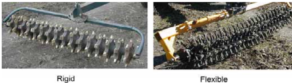
Figure 144: Examples of rigid and flexible rotary harrows
