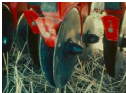
Figure 80: A rear view of a dedicated triple disc couler type furrow opener
