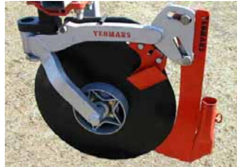
Figure 18: A plain disc coulters soil and residue cutting device
