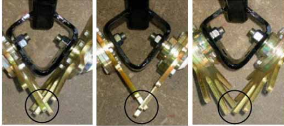
Figure 29: Top views of a finger wheel row preparation device showing the optional wheel positions
