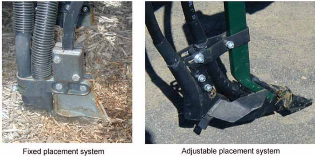
Figure 95: Fixed and adjustable seed and fertiliser placement systems for tine type opener
