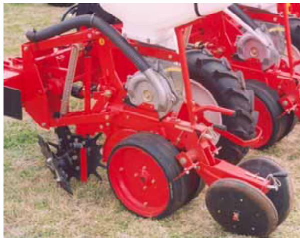
Figure 155: A planter utilising a 'dedicated gauge wheel' type of depth control
