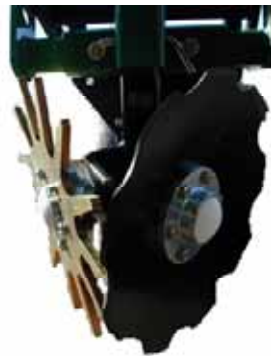
Figure 37: An example combined concave disc and single finger type row preparation device
