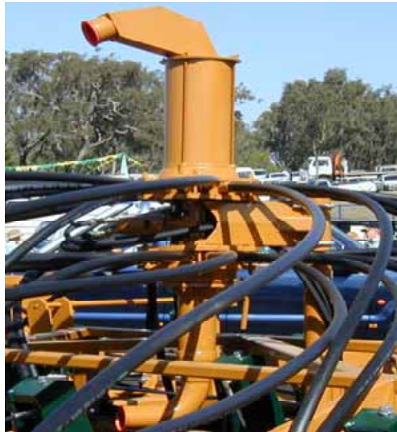
Figure 211: Seed and fertiliser heads incorporating hydraulically driven components
