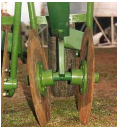
Figure 67: Opposed single compound angle disc coulters mounted on a common arm
