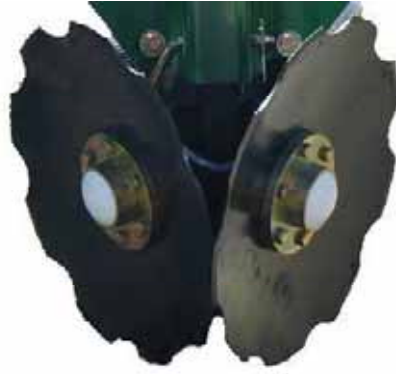
Figure 36: An example of a staggered, notched double
