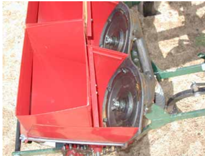
Figure 181: Twin inclined plate meters delivering seed to a common delivery tube
