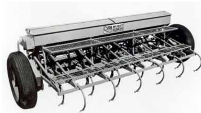
Figure 150: A drill planter utilising frame section gauging for furrow opener depth control
