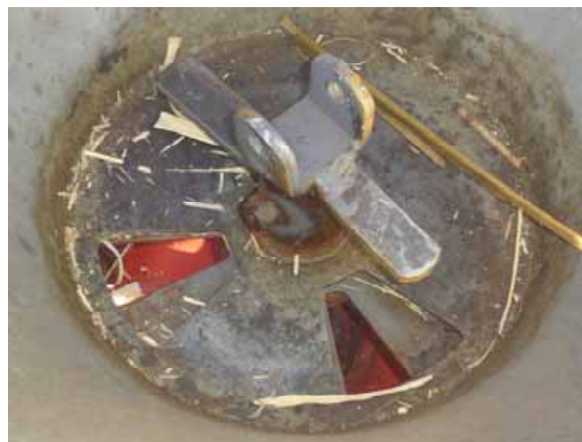
Figure 164: A stationary opening type seed meter using a sliding plate to adjust the outlet size
