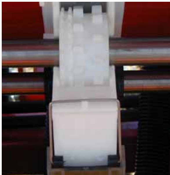
Figure 170: The rear view of a peg or studded external force feed seed metering system
