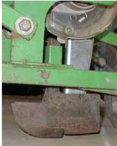
Figure 53: Seed delivery via a short dropper tube
