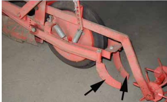
Figure 114: Opposed knife type covering devices
