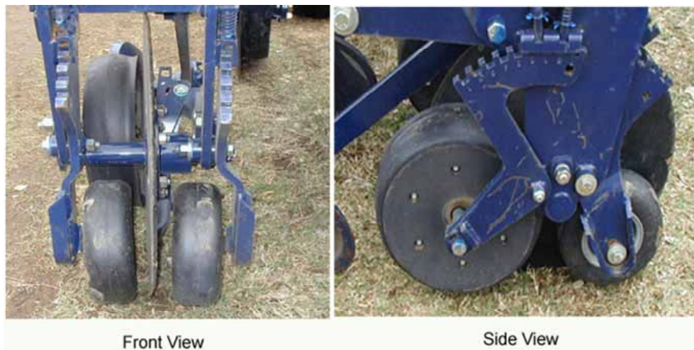
Figure 63: The front and side views of a single-angle disc coulters type furrow opener
