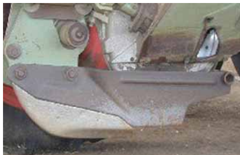
Figure 51: An example of a full runner type furrow opener
