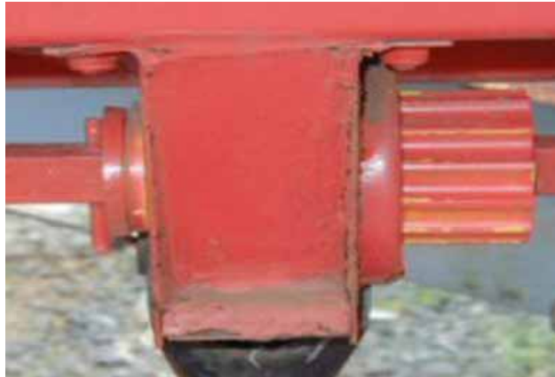
Figure 169: Front view of a fluted roller type seed meter
