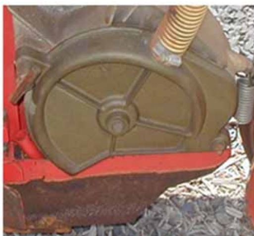
Side view of a vacuum disc seed meter
