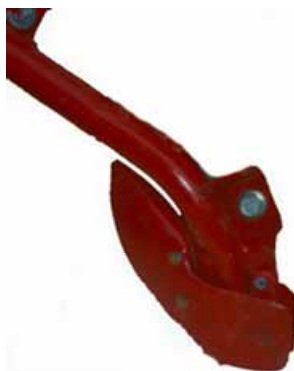
Figure 94: Rearward curved shoe type opener and seed placement device
