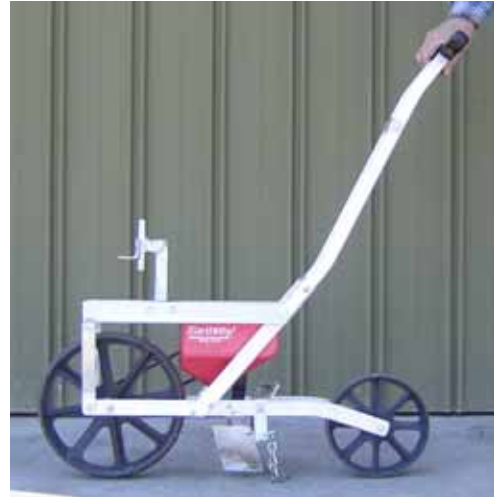
Figure 12: A single-row, hand-pushed, human-powered, precision planter
