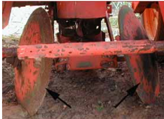
Figure 109: Rear view of a double concave disc type covering device
