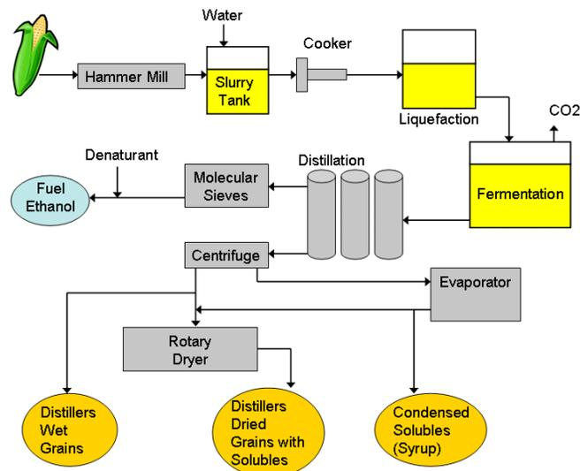
Figure 1. Conventional natural gas fired dry-grind ethanol process.
