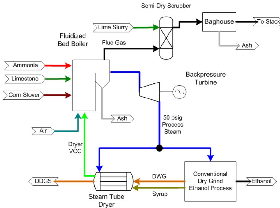
Figure 9. Corn stover combustion, level 2: CHP.
