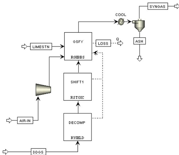
Figure 4. Aspen Plus model of fluidized bed gasification.
