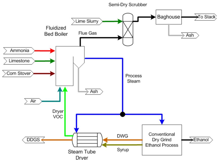
Figure 8. Corn stover combustion, level 1: Process heat only.
