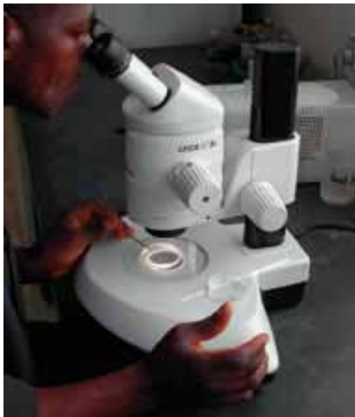
Using a dissection stereo-microscope with understage lighting.
