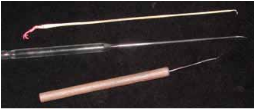
Figure 35. A sample of potential nematode picking tools: a bamboo splint; the tip of a pipette thinned using heat; dissection needle with an eyelash glued to the tip.
