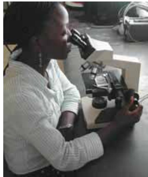
Using a compound stereo-microscope with understage lighting.
