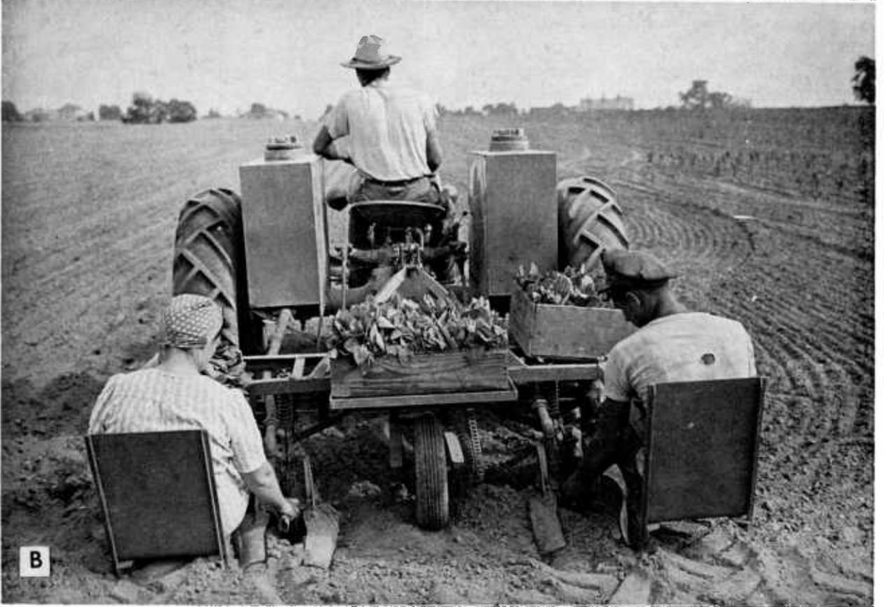
FIGURE 7.—Transplanting with tractor-drawn equipment: A , Single-row, power-lift transplanter used in setting burley tobacco in eastern Tennessee; B , two-row transplanter used in setting cigar filler plants in Pennsylvania.
