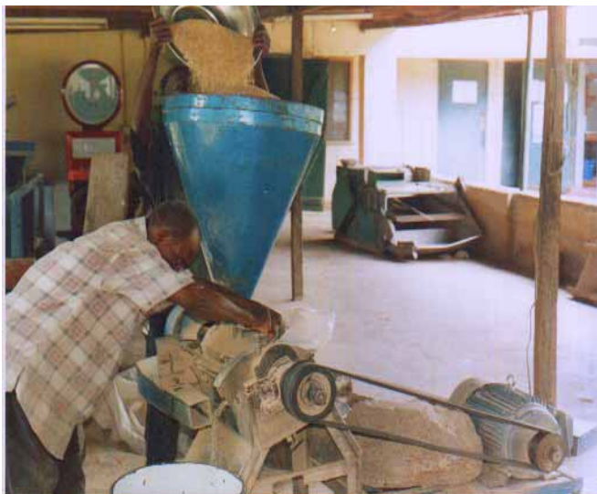
Plate 4: NCRI Fabricated Milling Machine
