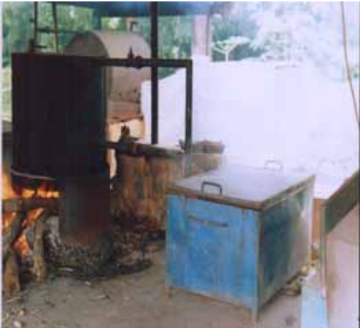
Plate 1: NCRI Parboiling System and the Drying Slab
